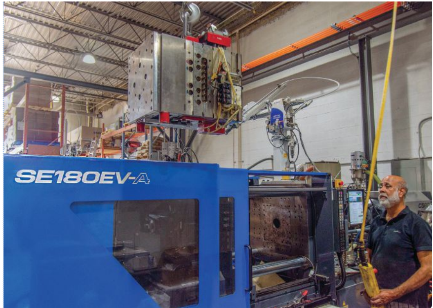
Average mold-change time is one metric Top Shops are measured on. Pictured here, Qualicase swapping out a tool. (Photo: Qualicase)
